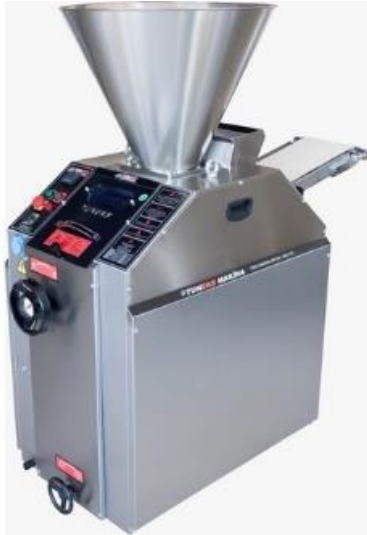
Picture 5: Dough cutting machine
