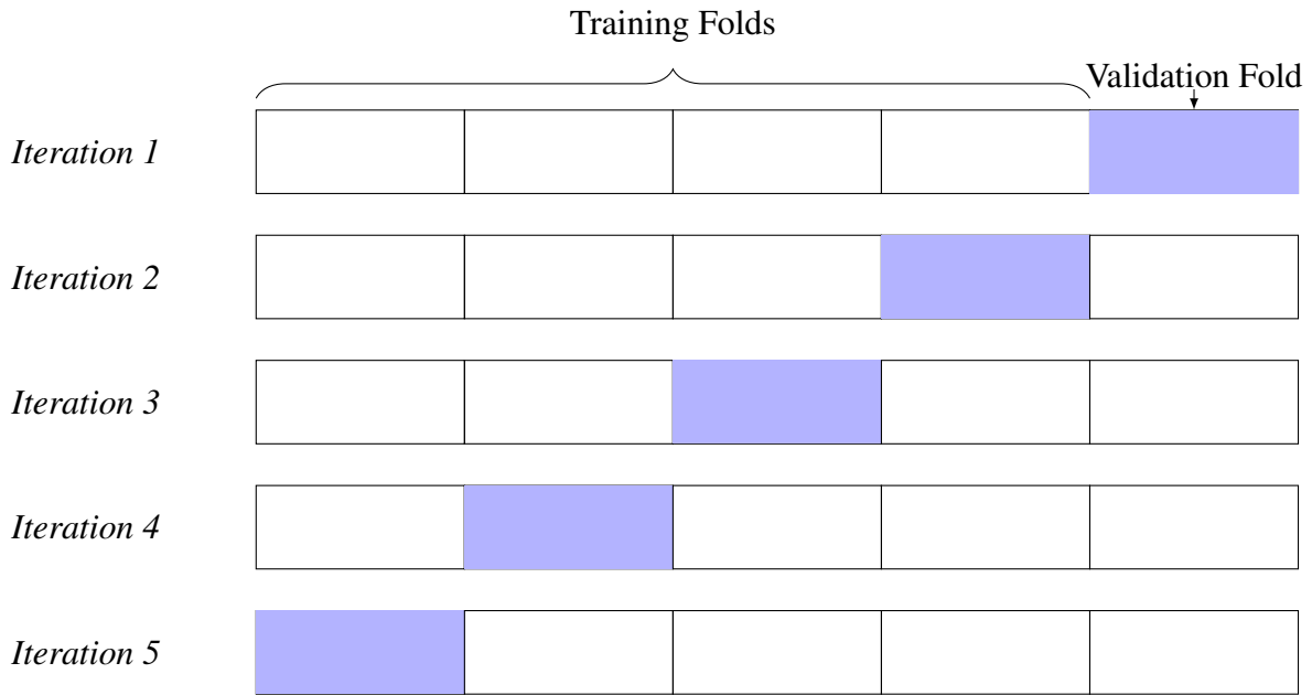
Figure 7: 5-Fold Cross-Validation Process. This diagram illustrates the 5-Fold Cross-Validation method used for model validation. In each iteration, the dataset is divided into 5 folds, where one fold is used for validation and the remaining folds are used for training. This process is repeated 5 times, with each fold being used as the validation set exactly once.
